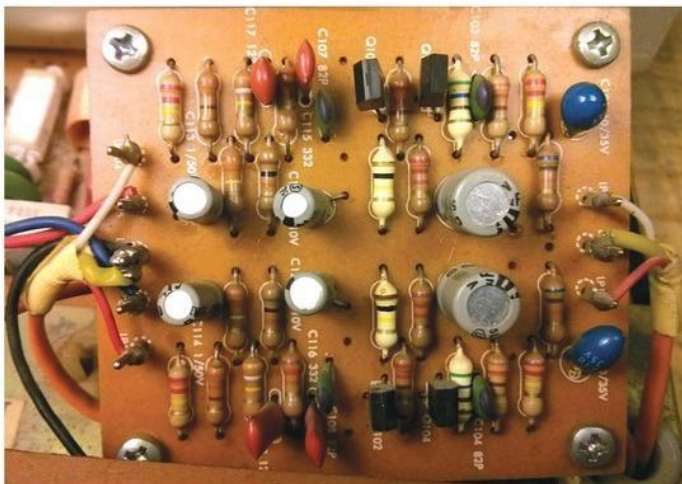
This phono amplifier PCB shows up in several other H/K amplifiers and receivers.
